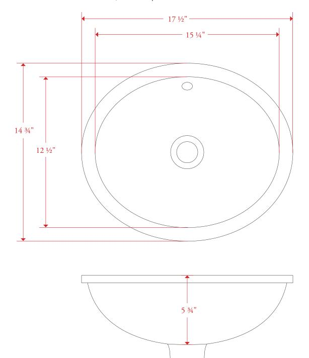
All measurements are in inches unless otherwise noted. Drawing shown at ¼ scale. Please do not scale drawing. Template is for reference only, not mortising purposes. All field cutting and fitting should be done with physical items. Porcelain bowls are fired and dimensions vary. Bowls are undermount, have an overflow, and fit a 1 ¼" drain (not included with bowl; included with purchase of basin set).
