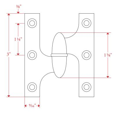
All measurements are in inches unless otherwise noted. Drawing shown at full scale. Left hand hinge shown; please specify hand when ordering. Template is for reference only, not mortising purposes.
