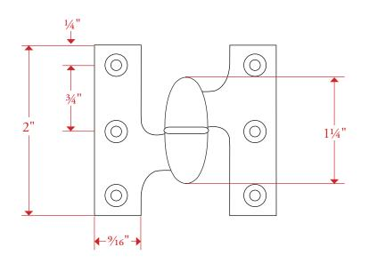
All measurements are in inches unless otherwise noted. Drawing shown at full scale. Left hand hinge shown; please specify hand when ordering. Template is for reference only, not mortising purposes. All field cutting and fitting should be done with physical hardware.
