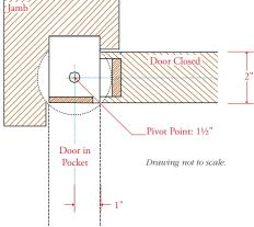
All measurements are in inches unless otherwise noted. Drawing shown at ¼ scale. Please do not scale drawing. Template is for reference only, not mortising purposes.
