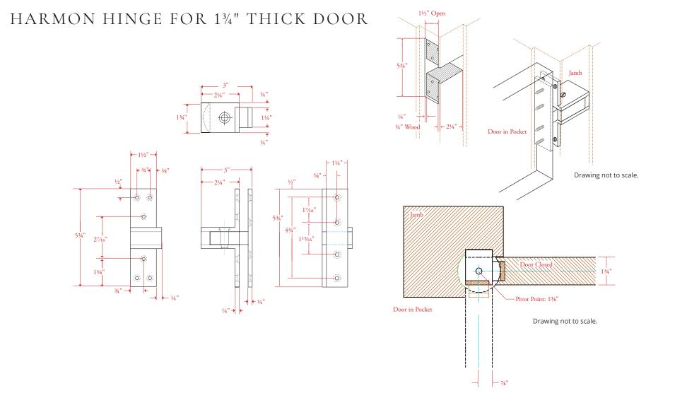
All measurements are in inches unless otherwise noted. Drawing shown at ¼ scale. Please do not scale drawing. Template is for reference only, not mortising purposes. All field cutting and fitting should be done with physical hardware. All harmon hinges are supplied with a positive stop. This hinge is handed; please specify right or left hand when ordering.
