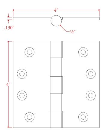
All measurements are in inches unless otherwise noted. Drawing shown at  $\frac{3}{4}$  to scale. Please do not scale drawing. Template is for reference only, not mortising purposes. All field cutting and fitting should be done with physical hardware.
