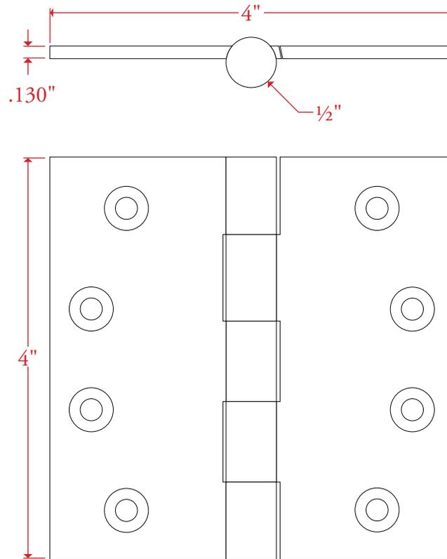
All measurements are in inches unless otherwise noted. Drawing shown at 3/4 to scale. Please do not scale drawing. Template is for reference only, not mortising purposes. All field cutting and fitting should be done with physical hardware.
