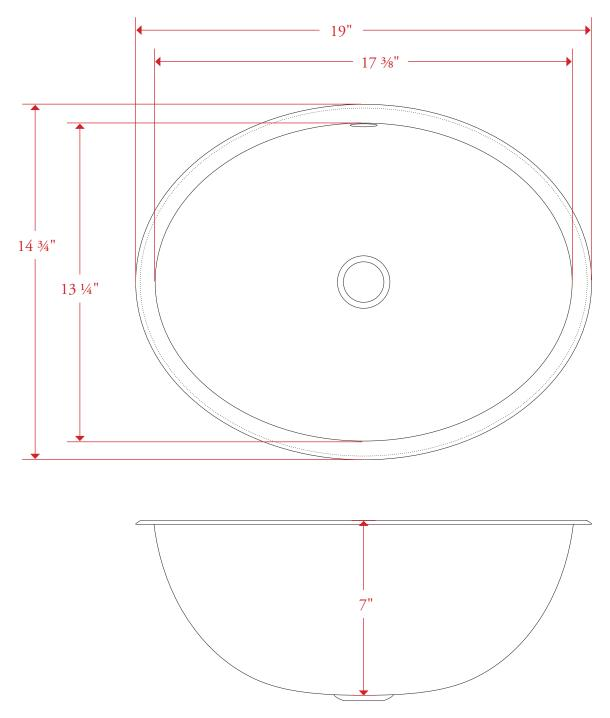
All measurements are in inches unless otherwise noted. Drawing shown at ½ scale. Please do not scale drawing. Template is for reference only, not mortising purposes. All field cutting and fitting should be done with physical items. Bowls are undermount, have an overflow, and fit a 1 ½" drain (not included with bowl; included with purchase of basin set).
