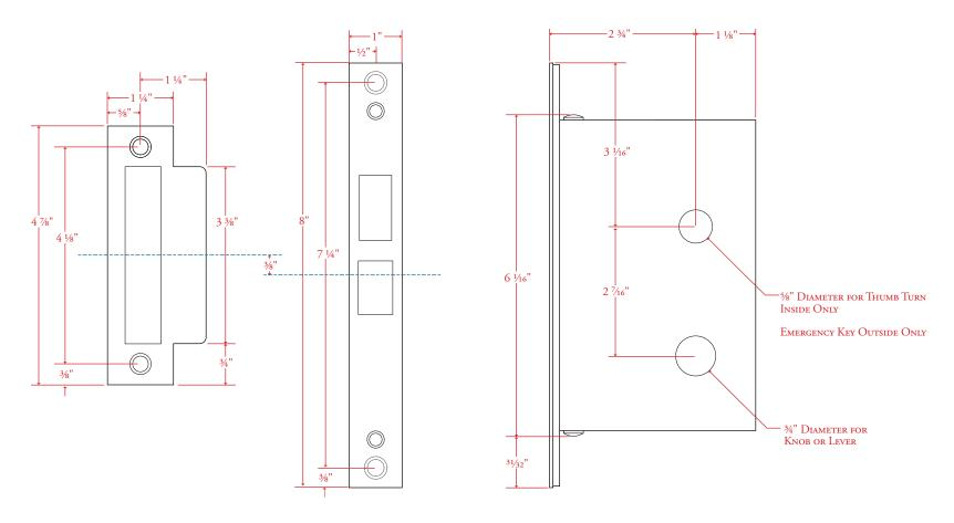
Drawing shown at ½ scale. Please do not scale drawing. Template is for reference only, not mortising purposes. All field cutting and fitting should be done with physical hardware.
