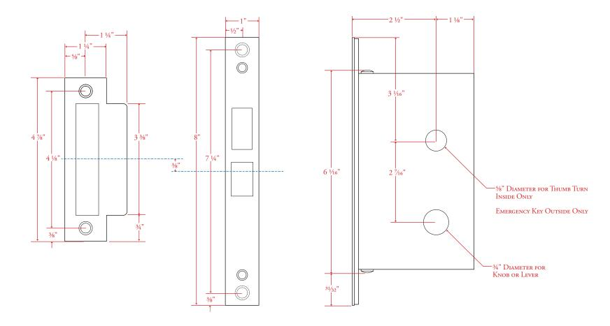
Drawing shown at ½ scale. Please do not scale drawing. Template is for reference only, not mortising purposes. All field cutting and fitting should be done with physical hardware. Please note when mounting hardware, face plate and strike use #12-24 flat head screws.
