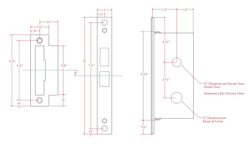
Drawing shown at ½ scale. Please do not scale drawing. Template is for reference only, not mortising purposes. All field cutting and fitting should be done with physical hardware. Please note when mounting hardware, face plate and strike use #12-24 flat head screws.
