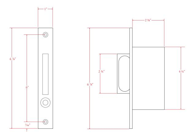
Drawing shown at ½ scale. Please do not scale drawing. Template is for reference only, not mortising purposes. All field cutting and fitting should be done with physical hardware. Please note when mounting hardware, face plate uses #7 flat head screws.
