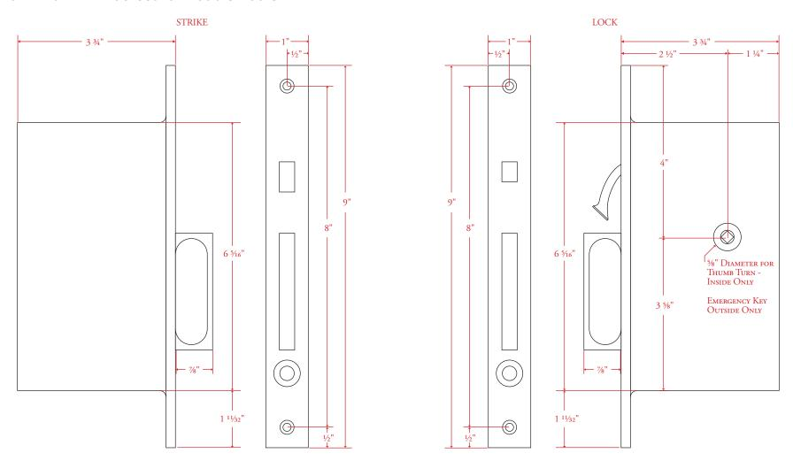
Drawing shown at  $\frac{1}{2}$  scale. Please do not scale drawing. Template is for reference only, not mortising purposes. All field cutting and fitting should be done with physical hardware.
