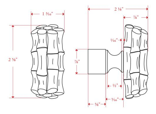
All measurements are in inches unless otherwise noted. Drawing shown at scale. Please do not scale drawing. Template is for reference only, not mortising purposes. All field cutting and fitting should be done with physical items.
