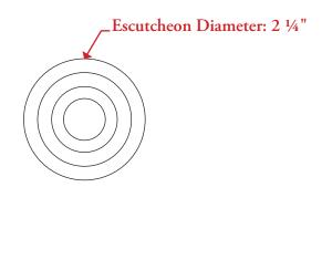
All measurements are in inches unless otherwise noted. Drawing shown at ½ scale. Please do not scale drawing. Template is for reference only, not mortising purposes.
