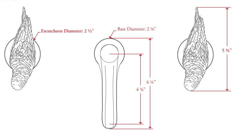
All measurements are in inches unless otherwise noted. Drawing shown at ½ scale. Please do not scale drawing. Template is for reference only, not mortising purposes. All field cutting and fitting should be done with physical hardware. Drilling Instructions: Hole sizes to be 1½" minimum for installation of valves and spout.
