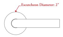
All measurements are in inches unless otherwise noted. Drawing shown at ½ scale. Please do not scale drawing. Template is for reference only, not mortising purposes. All field cutting and fitting should be done with physical hardware. All matching bathroom accessories are available. Drilling Instructions: Hole sizes to be 1 ½" minimum for installation of valves and spout.
