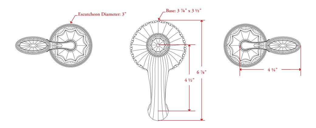
All measurements are in inches unless otherwise noted. Drawing shown at ½ scale. Please do not scale drawing. Template is for reference only, not mortising purposes.
