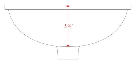
All measurements are in inches unless otherwise noted. Drawing shown at ¼ scale. Please do not scale drawing. Template is for reference only, not mortising purposes. All field cutting and fitting should be done with physical items. Porcelain bowls are fired and dimensions vary.
