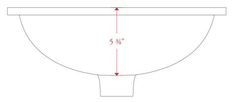
All measurements are in inches unless otherwise noted. Drawing shown at ¼ scale. Please do not scale drawing. Template is for reference only, not mortising purposes. All field cutting and fitting should be done with physical items. Porcelain bowls are fired and dimensions vary.
