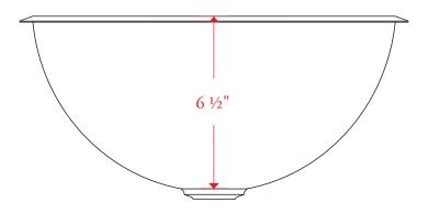
All measurements are in inches unless otherwise noted. Drawing shown at ¼ scale. Please do not scale drawing. Template is for reference only, not mortising purposes. All field cutting and fitting should be done with physical items. Bowls are undermount and fit a 1 ¼" drain (not included with bowl; included with purchase of basin set). Overflow not included; overflow can be added by request.
