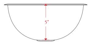
All measurements are in inches unless otherwise noted. Drawing shown at ¼ scale. Please do not scale drawing. Template is for reference only, not mortising purposes. All field cutting and fitting should be done with physical items. Bowls are undermount and fit a 1 ¼" drain (not included with bowl; included with purchase of basin set). Available with or without overflow; please specify when ordering.
